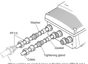
When working on conduit pipes or flexible pipes (PF1/2 only)  $$_{\rm F0405,EPS}$$
